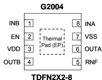
Note: Recommend connecting the Thermal Pad (EP) to the Ground for excellent power dissipation.
