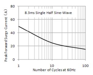
Figure 2.Maximum Non-Repetitive Peak Forward Surge Current
