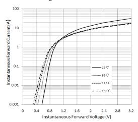
Figure 4. Typical Instantaneous Forward Characteristics
