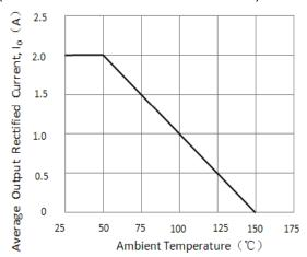
Figure 1. Forward Current Derating Curve
