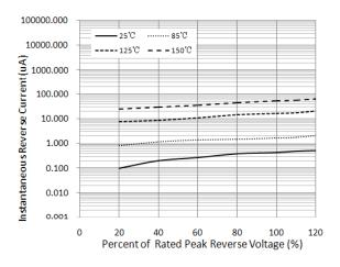
Figure 3. Typical Reverse Characteristics
