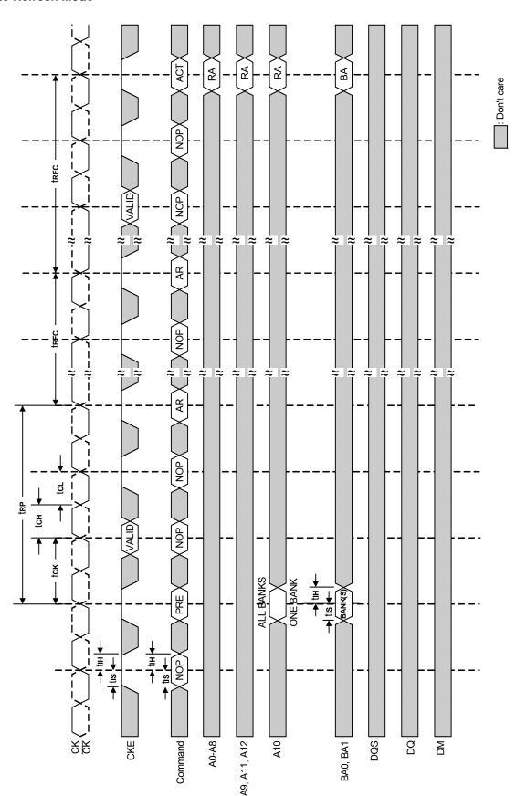
PRE = Precharge; ACT = Active; RA = Row address; BA = Bank address, AR = Autorefresh. NOP commands are shown for ease of illustration; other valid commands may be possible at these times. DM, DQ, and DQS signals are all don't care/high-Z for operation shown.
