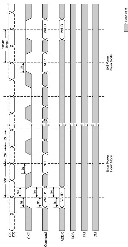
\* = If this command is a Precharge (or if the device is already in the idle state) then the power down mode shown is Precharge power down. If this command is an Active (or if at least one row is already active), then the power down mode No column access are allowed to be in progress at the time power down is entered.
