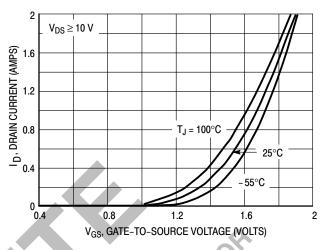
Figure 2. Transfer Characteristics
