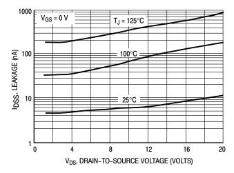
Figure 6. Drain-To-Source Leakage Current versus Voltage
