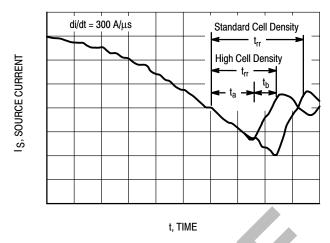
Figure 11. Reverse Recovery Time (t<sub>rr</sub>)
