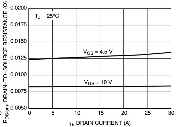
Figure 4. On-Resistance vs. Drain Current and Gate Voltage
