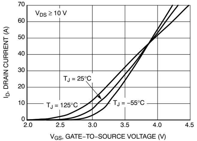
Figure 2. Transfer Characteristics
