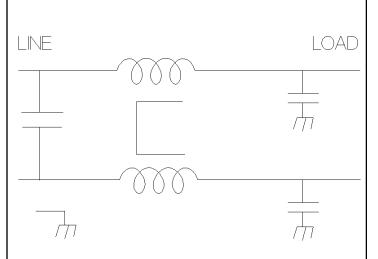
Diel. Withstanding (Line—GND) = \_\_\_\_\_1500 VDC; 1 Min Diel. Withstanding (Line—Line) = \_\_\_\_\_1500 VDC; 1 Min
