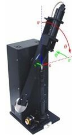
Goniometer coordinate system
