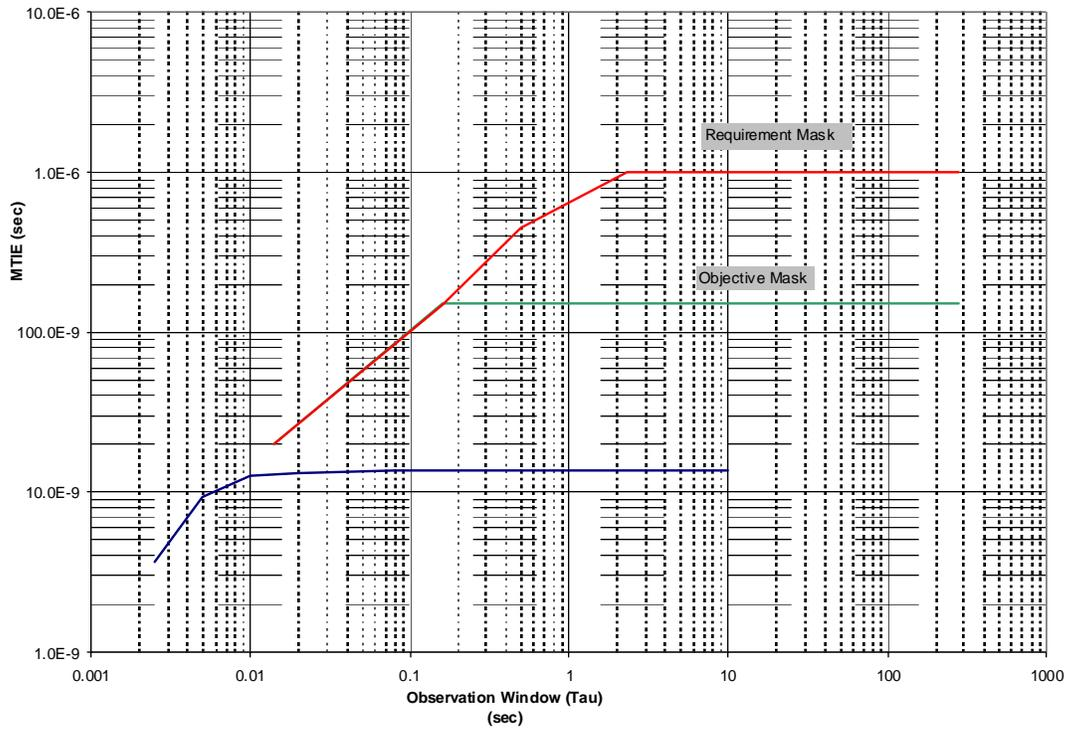
**\*NOTE:** The wider bandwidth of this model may result in a break in the GR-253-CORE, R5-135 Switching Mask for observation times of <50ms.
