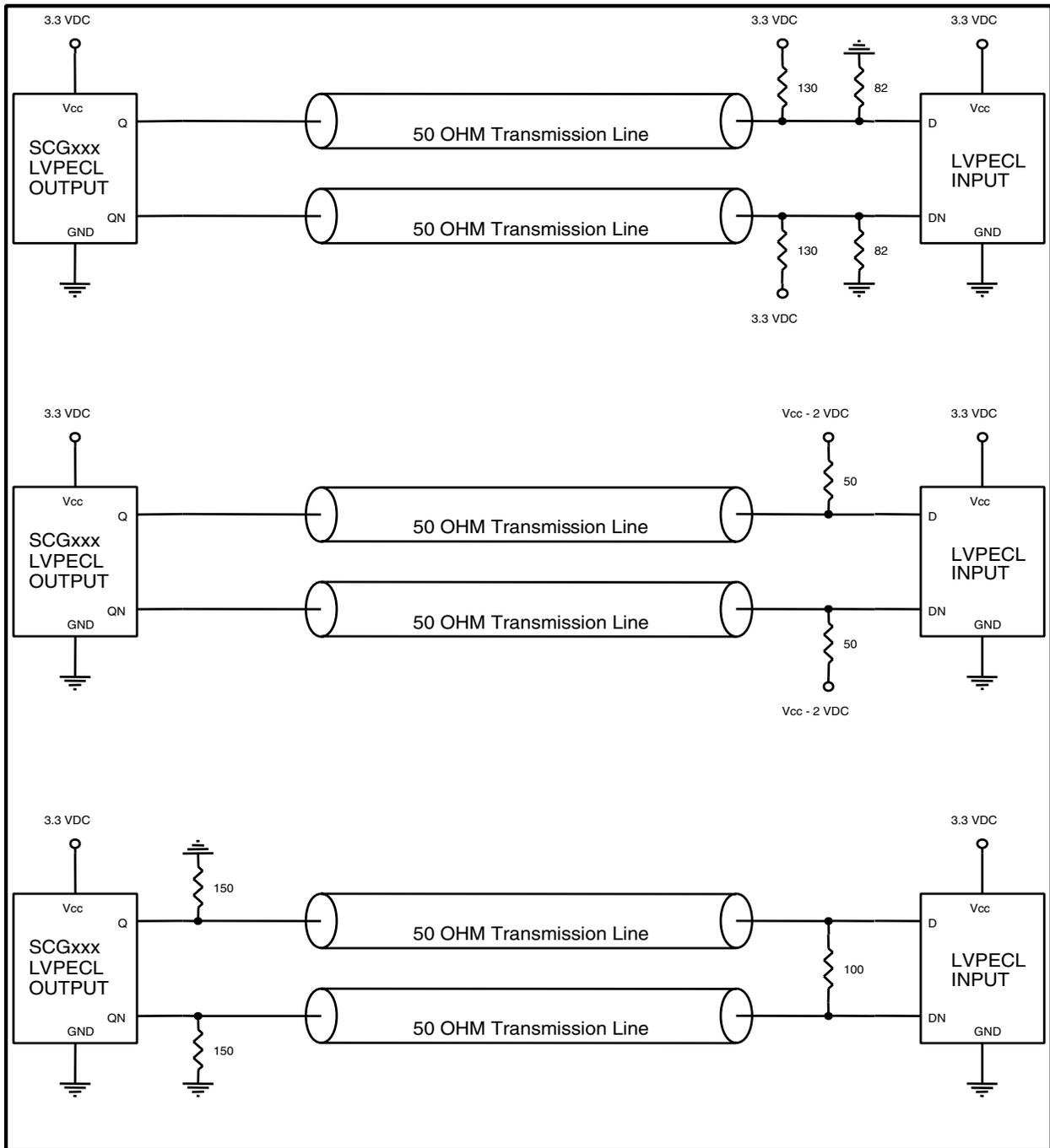
If PECL outputs do not drive a long line (< 0.5"), a single 150Ω termination resistor to ground may be used for each pin.
