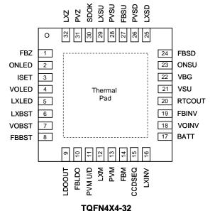
Note: Recommend connecting the Thermal Pad to the Ground for excellent power dissipation.
