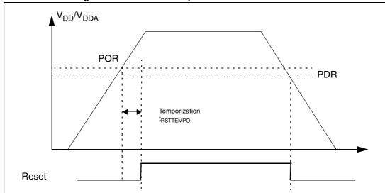
Figure 5. Power on reset/power down reset waveform
