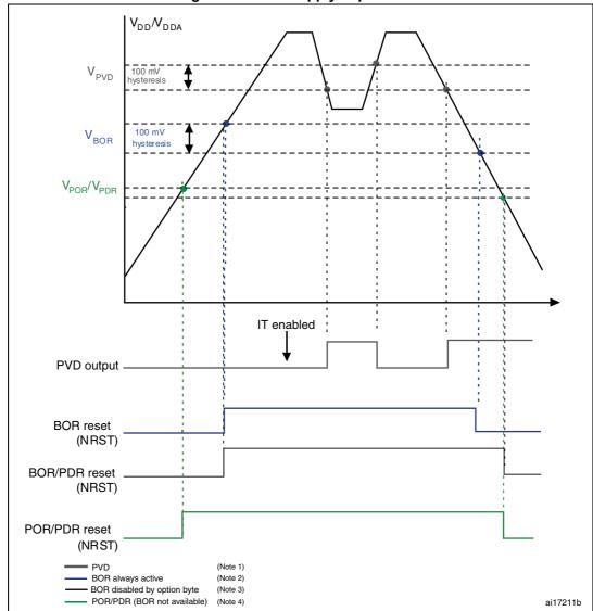
Figure 4. Power supply supervisors
