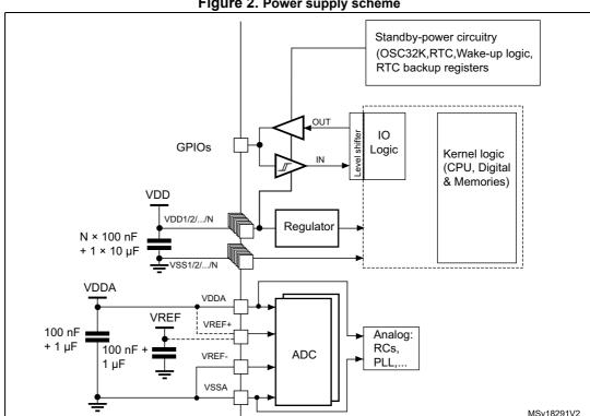
Figure 2. Power supply scheme
