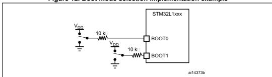
Figure 12. Boot mode selection implementation example
