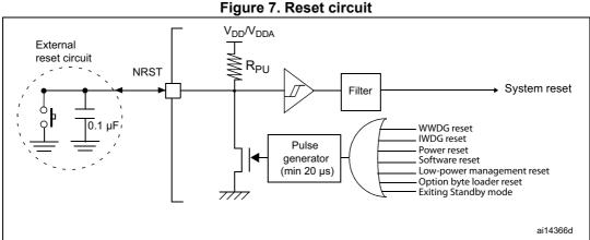
The STM32L does not require an external reset circuit to power-up correctly. Only a pull-down capacitor is recommended to improve EMS performance by protecting the device
