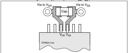
Figure 15. Typical layout for V<sub>DD</sub>/V<sub>SS</sub> pair
