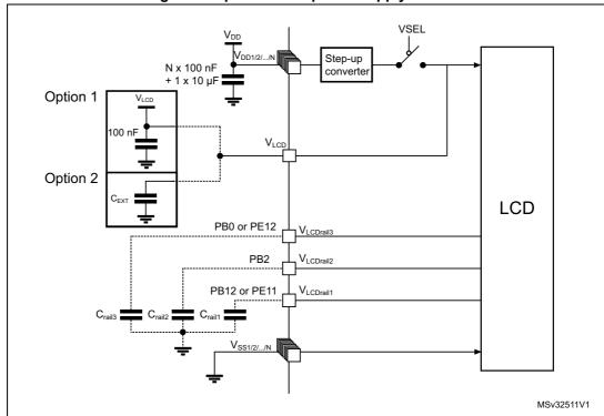
Figure 3. Optional LCD power supply scheme
