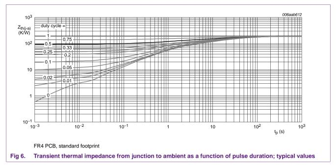
Approximate the  $Z_{th(j-a)}$  value from the graph at  $\delta$  = 0.5 and calculate the maximum power dissipation with the formula:
