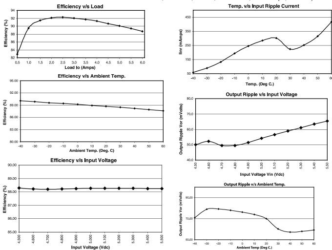
NOTE: The ambient temperature is as measured at approx. 1/4" away on the back side of the unit, with the probe end at approx. center (vertical & horizontal). For thermal performance, the unit was mounted on a 4"x4" PCB (with ground plane) & enclosed in a box so that it operates in a controlled environment.
