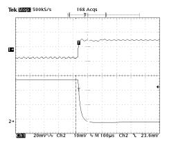
Operating conditions are as follows: Vin=5V, Vo=3.3V, Load change from Io=100% to Io=0%, TA=25°C, Cin=100 $\mu$ F, Co=0.
