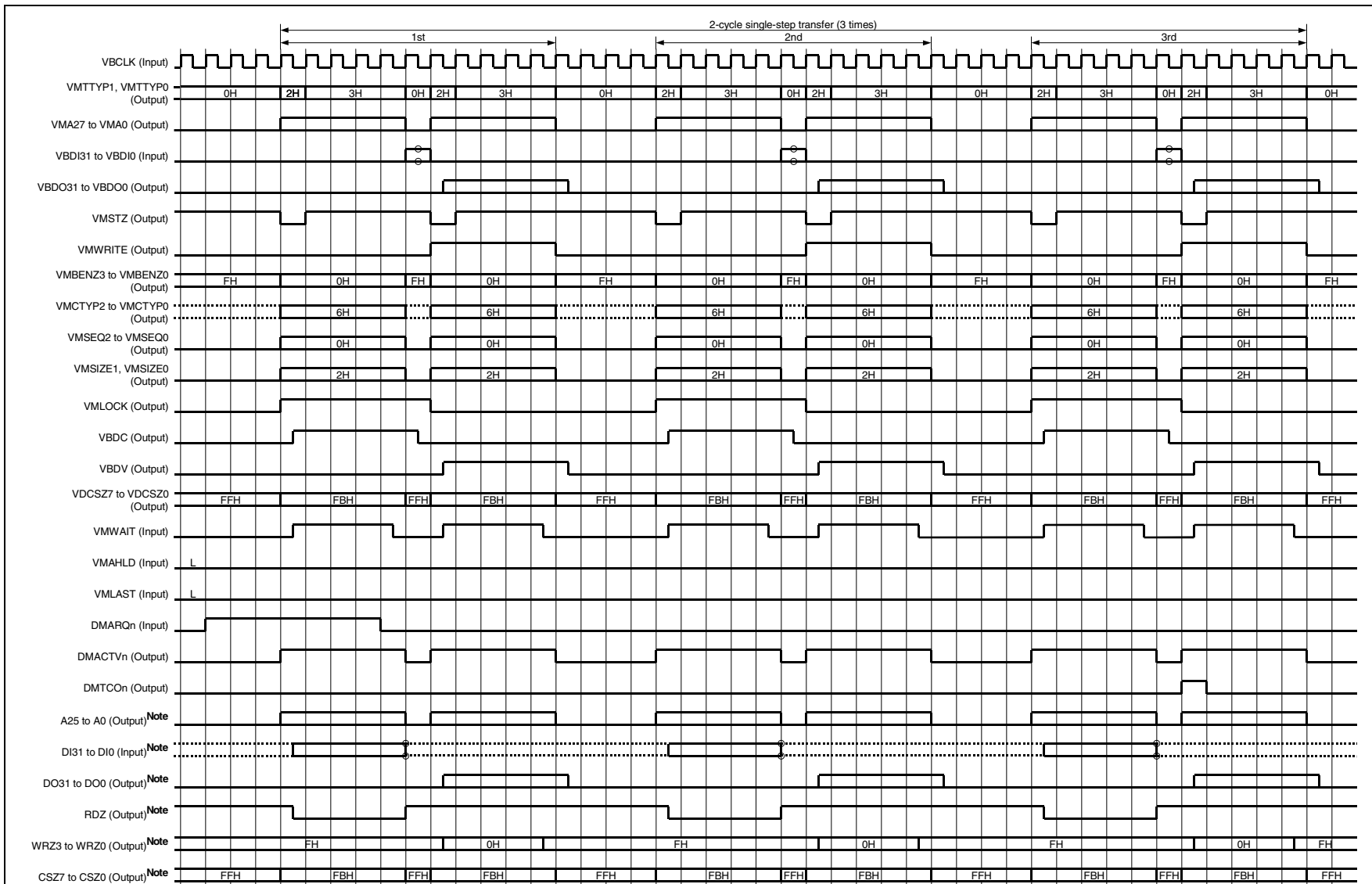
Figure 7-31. Example of Two-Cycle Single-Step Transfer Timing (Between External SRAMs Connected to NT85E500)
