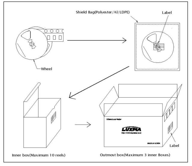
• The LEDs are packed in cardboard boxes after taping. The label shows part number, lot number, rank, and quantity.
