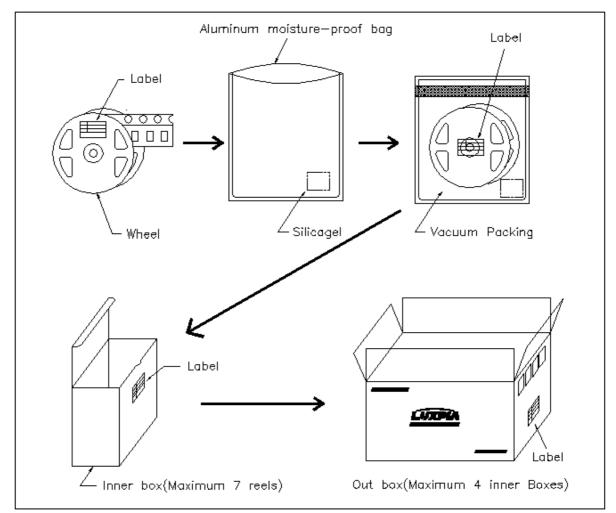
• The LEDs are packed in cardboard boxes after taping. The label shows part number, lot number, rank, and quantity.
