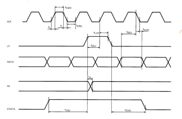
Test Conditions (Unless Otherwise Noted, V<sub>DD</sub> = 5.0 V ± 10%, V<sub>SS</sub> = 0 V, Ta = -20 to 70°C)
