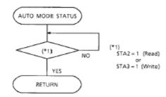
Note 4: When using the MSB = 0 command, a Status Read must be performed.
