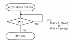
Note 4: When using the MSB = 0 command, a Status Read must be performed.
