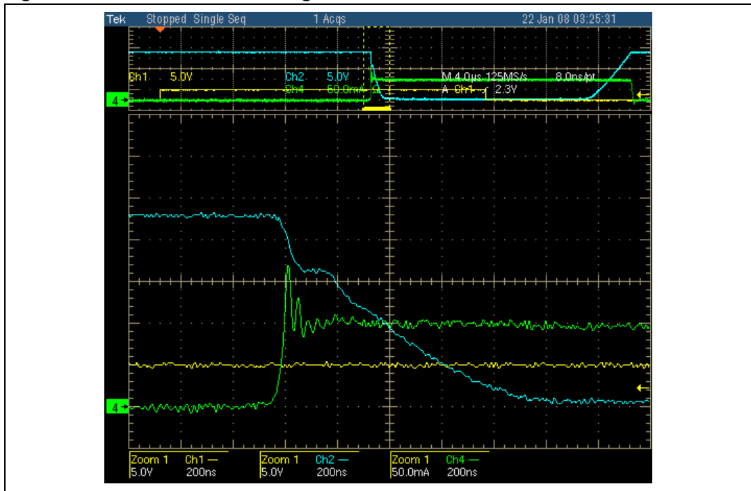
Figure 9. Low-side switch configuration turn-on behavior (1)
