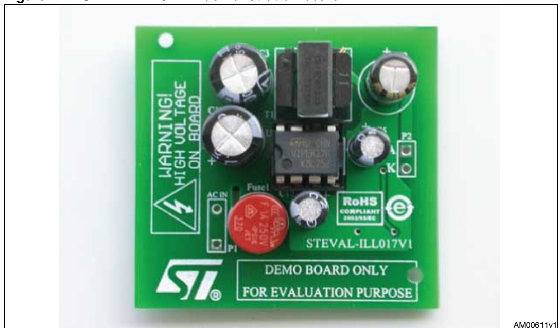
Figure 1. STEVAL-ILL017V1 demonstration board
