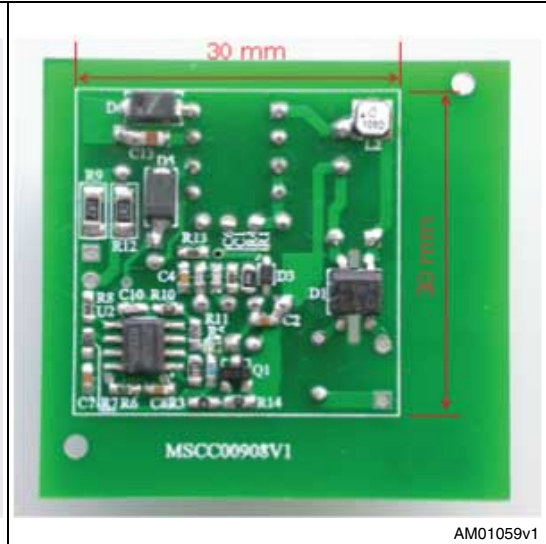
Figure 7. Bottom view with SMD parts
