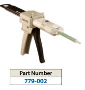
Twin push-rod 1:1 ratio epoxy dispensing gun for use with duo syringe epoxy and mixing nozzle sold separately. Durable heavy-duty plastic. Gun type hand grip with ratcheting trigger to advance push-rods.
