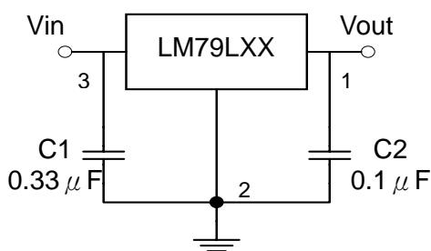
A common ground is required between the input and the output voltages. The input voltage must remain typically 2.0V above the output voltage even during the low point on the input ripple voltage.
