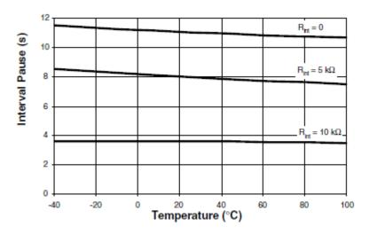
Figure 5. After-wiping Time = f (T);  $C_t$  = 22  $\mu$ F;  $V_{Batt}$  = 8 V
