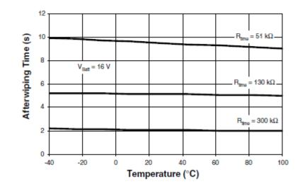
Figure 7. After-wiping Time = f (T);  $C_t$  = 22  $\mu$ F;  $V_{Batt}$  = 16 V
