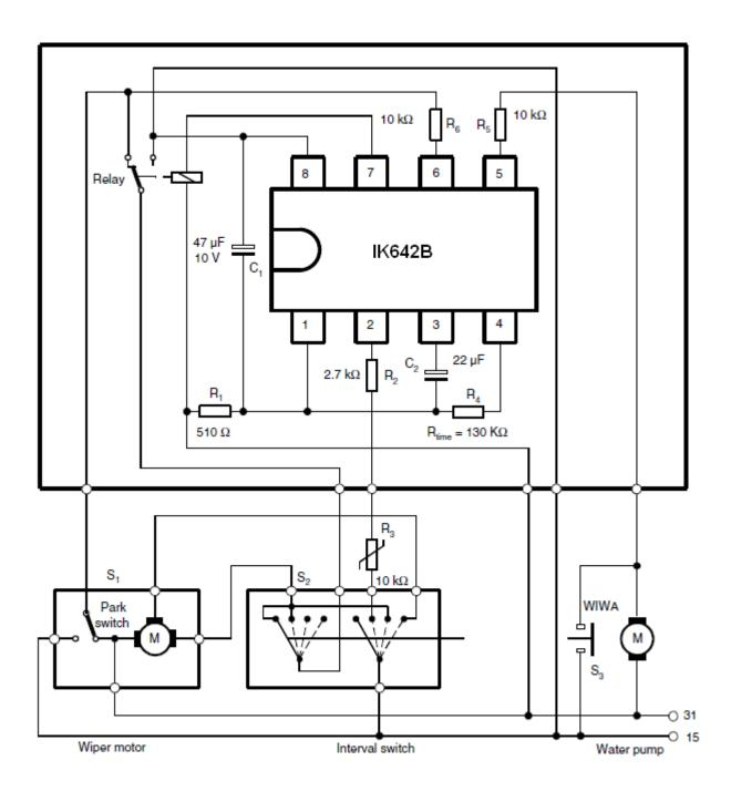
Figure 3. Application Circuit with Interval and Wipe/Wash Operation
