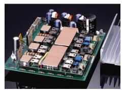
Gap Pad® VO Soft is recommended for applications that require a minimum amount of pressure on components. Gap Pad® VO Soft is a highly conformable, low-modulus, filled-silicone polymer on a rubber-coated fiberglass carrier. The material can be used as an interface where one side is in contact with a leaded device.
