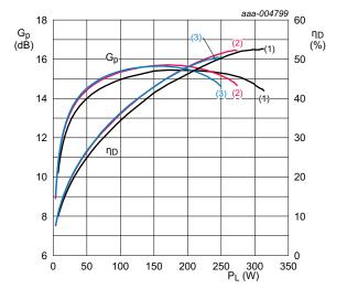
$V_{DS} = 28 \text{ V}; I_{Dq} = 20 \text{ mA}.$
