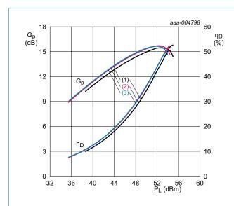
$V_{DS}$  = 28 V;  $I_{Dq}$  = 20 mA.
