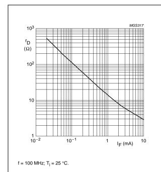
Fig.2 Forward resistance as a function of the forward current; typical values.
