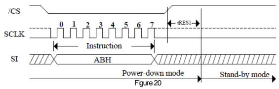
Figure 21 Release Power-Down/Read Device ID Sequence Diagram
