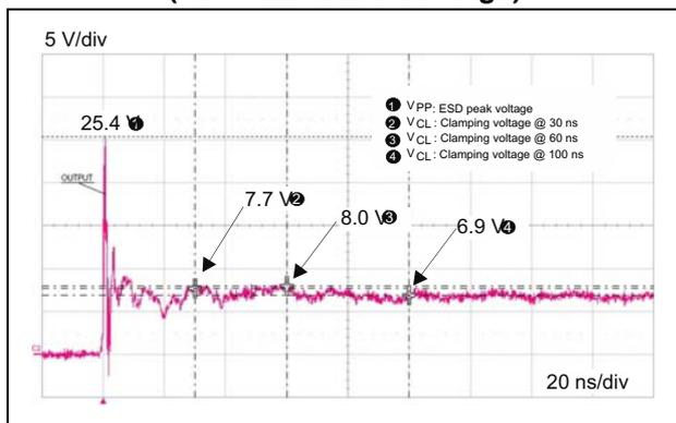
Figure 8. ESD response to IEC 61000-4-2 (-8 kV contact discharge)
