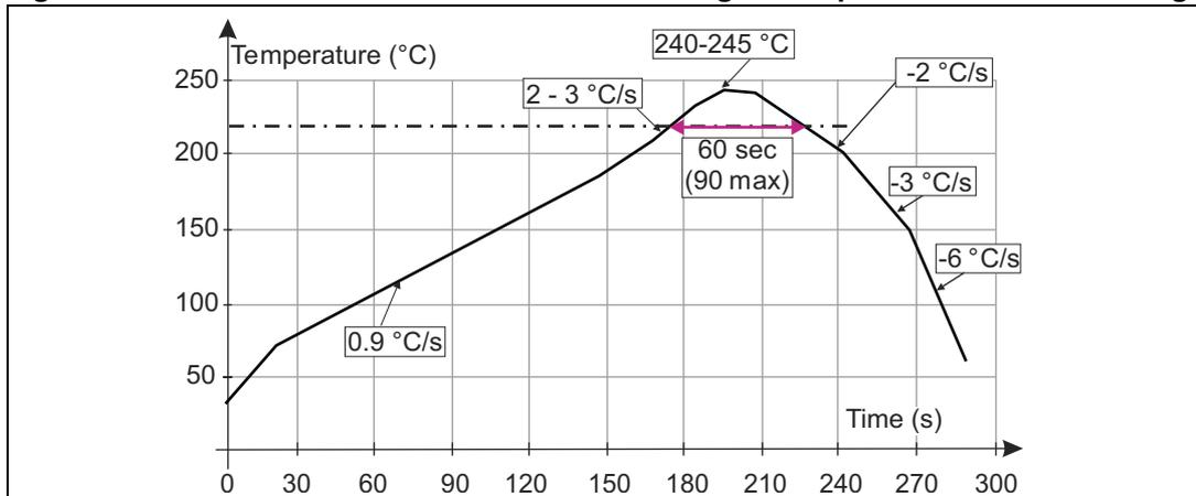
Note: Minimize air convection currents in the reflow oven to avoid component movement.
