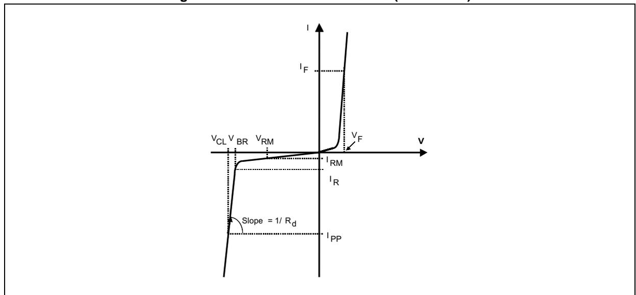
**Table 2. Electrical characteristics (values,  $T_{amb} = 25\text{ °C}$ )**
