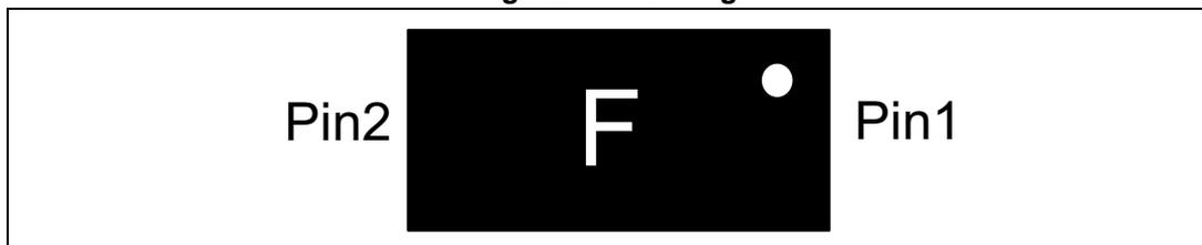
Note: Product marking may be rotated by multiples of 90° for assembly plant differentiation. In no case should this product marking be used to orient the component for its placement on a PCB. Only pin 1 mark is to be used for this purpose.
