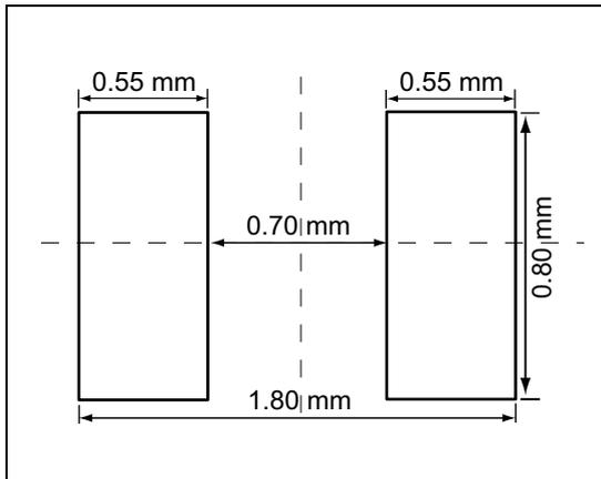
Figure 11. Alternative footprint, dimensions in mm
