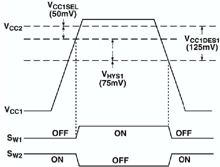
Figure 1. Supply Threshold Diagram
