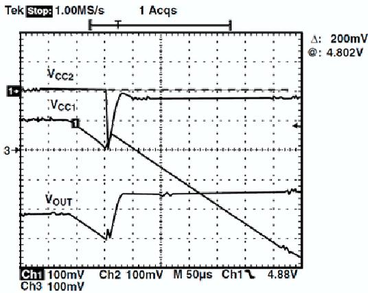
Figure 8.  $V_{CC1}$  Falling form 0 V to 5 V ( $V_{CC2} = 5$  V).
