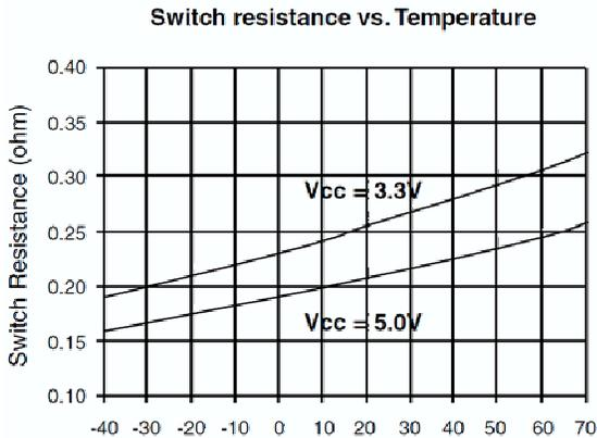
Figure 3. Switch Resistance vs. V<sub>CC</sub> with Temperature
