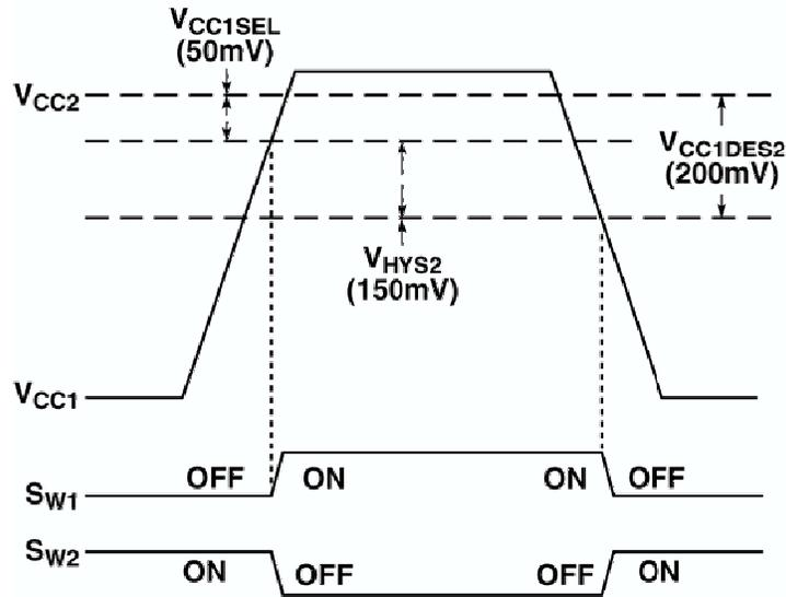
Figure 2. Supply Threshold Diagram
