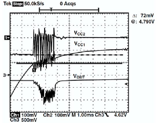
Figure 9.  $V_{CC1}$  Rising ( $V_{CC2}@ = 5$  V).
