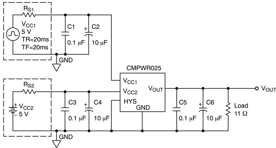
**Figure 6. Transient Characterization Test Set-Up**
