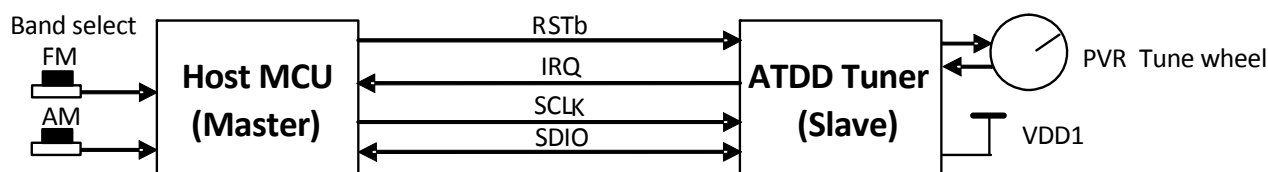
Figure 5. Band Detection and Control by System Controller
