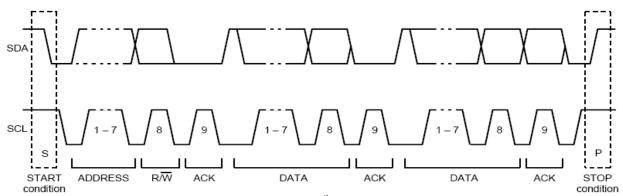
Fig. 11-2: RW bit in the 8<sup>th</sup> bit after IIC address
