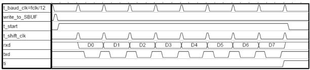
Fig. 7-1: Transmit mode 0 for Serial 0
