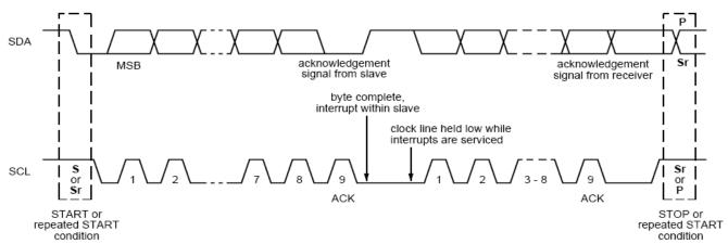
Fig. 11-1: Acknowledgement bit in the 9<sup>th</sup> bit of a byte transmission
