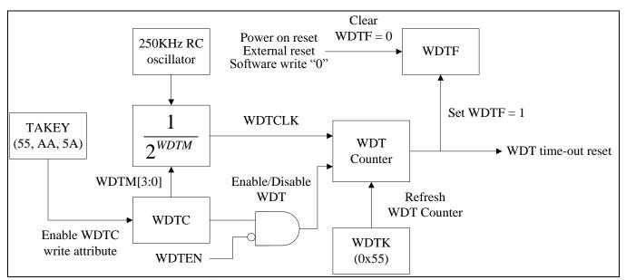
Fig. 8-1: Watchdog timer block diagram
