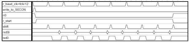
Fig. 7-2: Receive mode 0 for Serial 0
