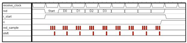
Fig. 7-4: Receive mode 1 for Serial 0
