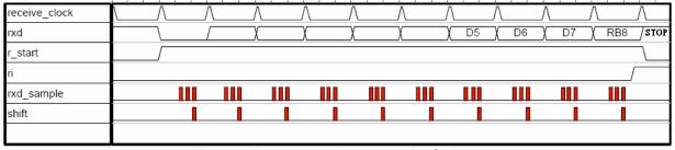
Fig. 7-6: Receive modes 2 and 3 for Serial 0
