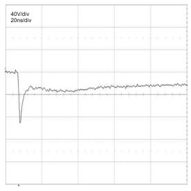
Figure 2 IEC 6100-4-2 Clamping Voltage -8kV Contact
