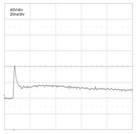
Figure 1 IEC 6100-4-2 Clamping Voltage +8kV Contact
