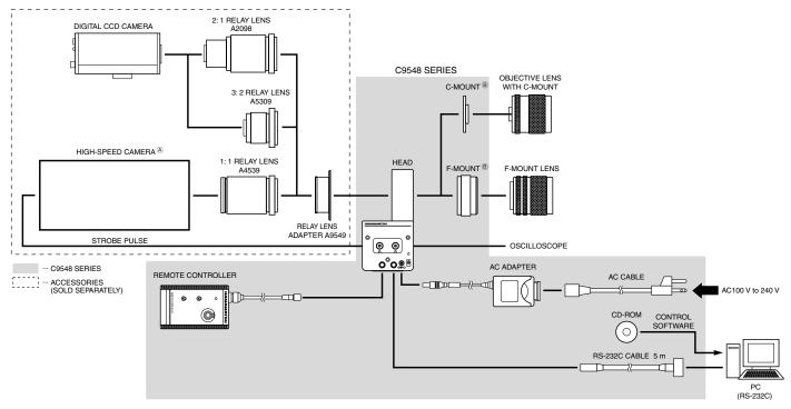
NOTE: (a) Connection to a high-speed camera may not be possible depending on the readout frame rate. Always consult us before placing an order.
