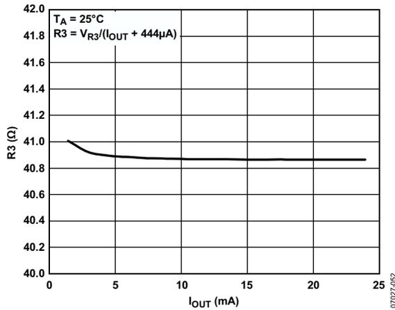
Figure 50. R3 Resistor Value vs. I<sub>OUT</sub>
