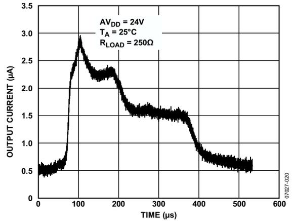
Figure 23. Output Current vs. Time on Power-Up
