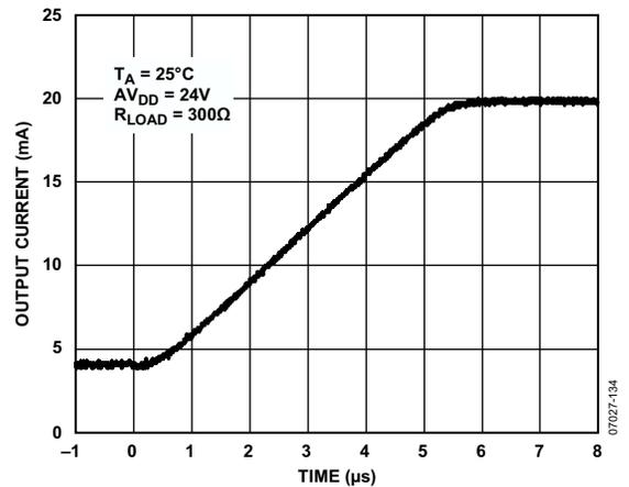
Figure 36. 4 mA to 20 mA Output Current Step
