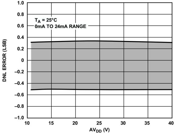
Figure 19. Differential Nonlinearity Error vs.  $AV_{DD}$ , Internal  $R_{SET}$
