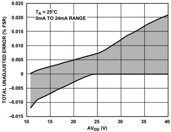
Figure 20. Total Unadjusted Error vs.  $AV_{DD}$ , External  $R_{SET}$
