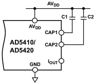
Figure 44. I<sub>out</sub> Filtering Capacitors
