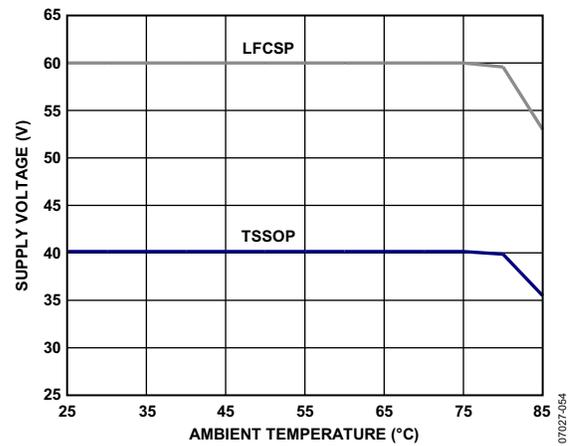
Figure 54. Maximum Supply Voltage vs. Ambient Temperature
