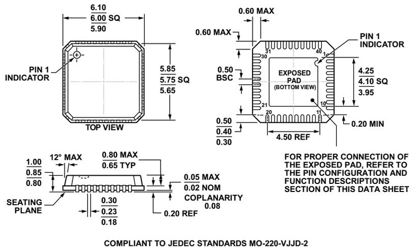
Figure 57. 40-Lead Lead Frame Chip Scale Package [LFCSP\_VQ] 6 mm x 6 mm Body, Very Thin Quad (CP-40-1)
