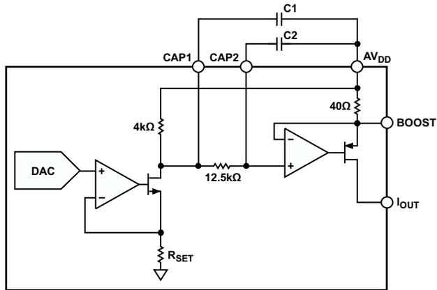
Figure 45. I<sub>out</sub> Filter Circuitry
