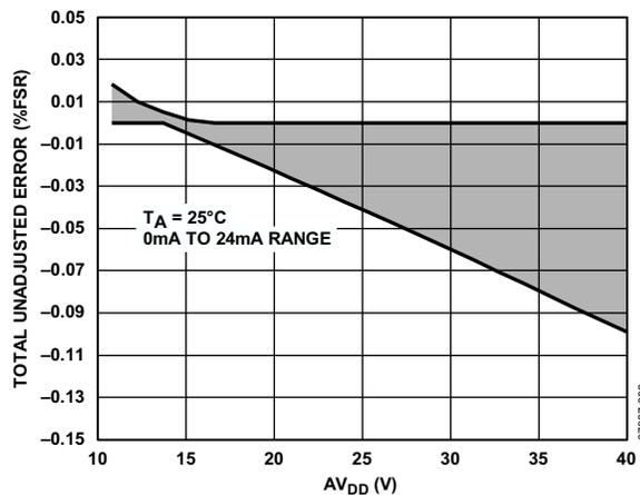
Figure 21. Total Unadjusted Error vs.  $AV_{DD}$ , Internal  $R_{SET}$
