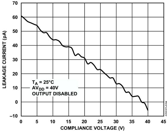
Figure 31. Output Leakage Current vs. Compliance Voltage
