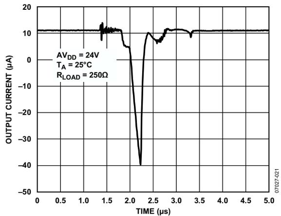
Figure 24. Output Current vs. Time on Output Enable
