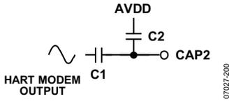
Figure 42. Coupling HART Signal
