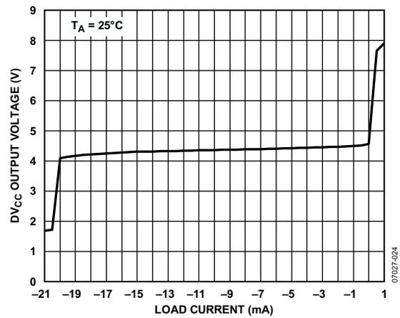
Figure 27.  $DV_{CC}$  Output Voltage vs. Load Current
