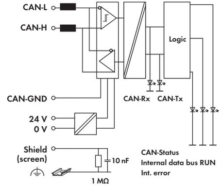
The CAN Gateway supports CAN Layer 2, while meeting CAN specifications 2.0A (11-bit identifier) and 2.0B (29-bit identifier). Function blocks allow the gateway to read and write higher-protocol telegrams (e.g., CANopen).
