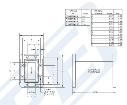
WR-137 Commercial Grade Straight Waveguide Section 6 Inch Length with CPR-137G Flange Operating from 5.85 GHz to 8.2 GHz from Pasternack Enterprises has same day shipment for domestic and International orders. Our RF, microwave and millimeter wave products maintain a 99% availability and are part of the broadest selection in the industry.
