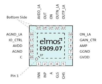
Fig. 2: Package Pinout E909.07 (Top View)
