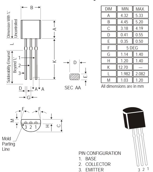
The TO-92 Package, Tape and Ammo Pack Drawings are correct as on the date of issue/revision of this Data Sheet.
