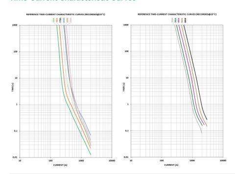
All ZCase Starters T/C curves were performed on the left or right side of the metal bar as shown in pictures above. A 50mm<sup>2</sup> Cu wire was mounted at the mid hole (M8) of the metal bar as current feed.
