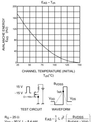
$$E_{AS} = \frac{1}{2} \cdot L \cdot I^2 \cdot \left( \frac{B_{VDSS}}{B_{VDSS} - V_{DD}} \right)$$
