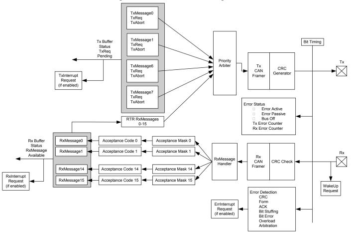
Figure 7-15. CAN Controller Block Diagram
