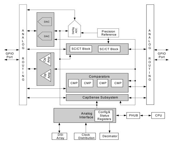
Figure 8-1. Analog Subsystem Block Diagram
