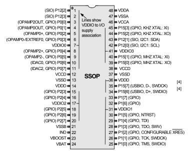
Figure 2-3. 48-pin SSOP Part Pinout
