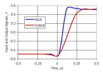
Figure 11-28. Opamp Step Response, Falling
