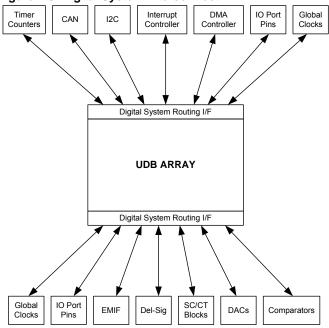
Interrupt and DMA routing is very flexible in the CY8C34 programmable architecture. In addition to the numerous fixed function peripherals that can generate interrupt requests, any data signal in the UDB array routing can also be used to generate a request. A single peripheral may generate multiple independent interrupt requests simplifying system and firmware design. Figure 7-10 shows the structure of the IDMUX (Interrupt/DMA Multiplexer).
