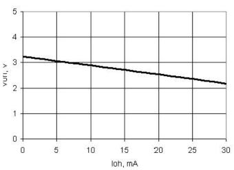
Figure 11-19. USBIO Output Low Voltage and Current, GPIO Mode
