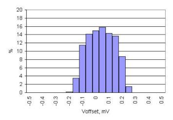
Figure 11-22. Opamp Voffset vs Temperature,  $V_{DDA} = 5V$
