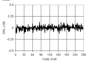
Figure 11-35. IDAC DNL vs Temperature, Range = 255  $\mu$ A, High speed mode
