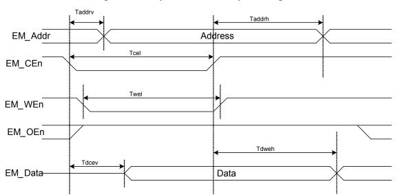
Figure 11-61. Asynchronous Write Cycle Timing
