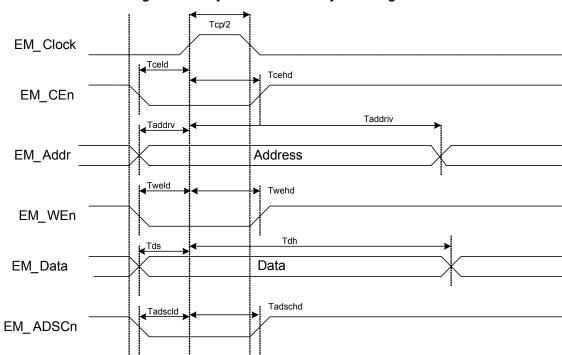
Figure 11-63. Synchronous Write Cycle Timing
