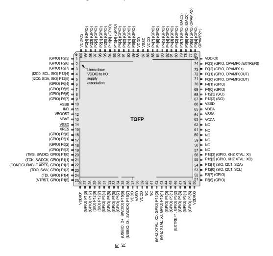
Figure 2-6. 100-pin TQFP Part Pinout
