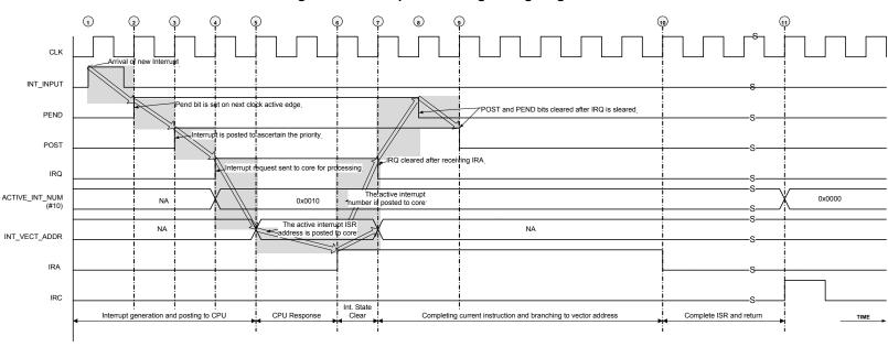
Figure 4-2. Interrupt Processing Timing Diagram
