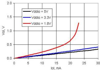
Figure 11-15. SIO Output High Voltage and Current, Regulated Mode
