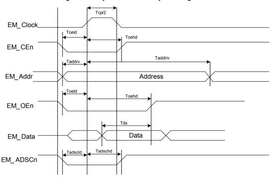
Figure 11-62. Synchronous Read Cycle Timing
