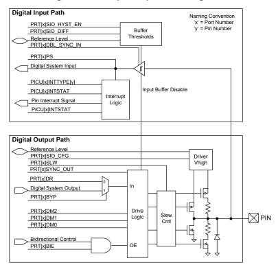
Figure 6-9. SIO Input/Output Block Diagram
