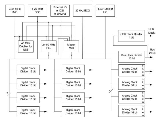
Figure 6-1. Clocking Subsystem
