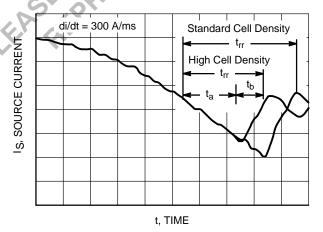
Figure 11. Reverse Recovery Time (t<sub>rr</sub>)
