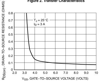
Figure 3. On-Resistance versus Gate-To-Source Voltage
