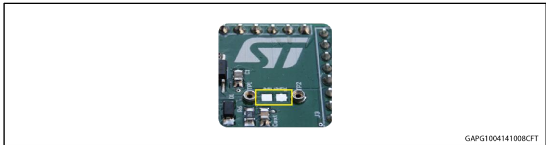
Figure 5: Pads for soldering SMD resistor
