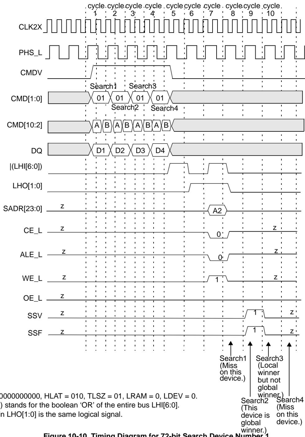
**Figure 10-10. Timing Diagram for 72-bit Search Device Number 1**
