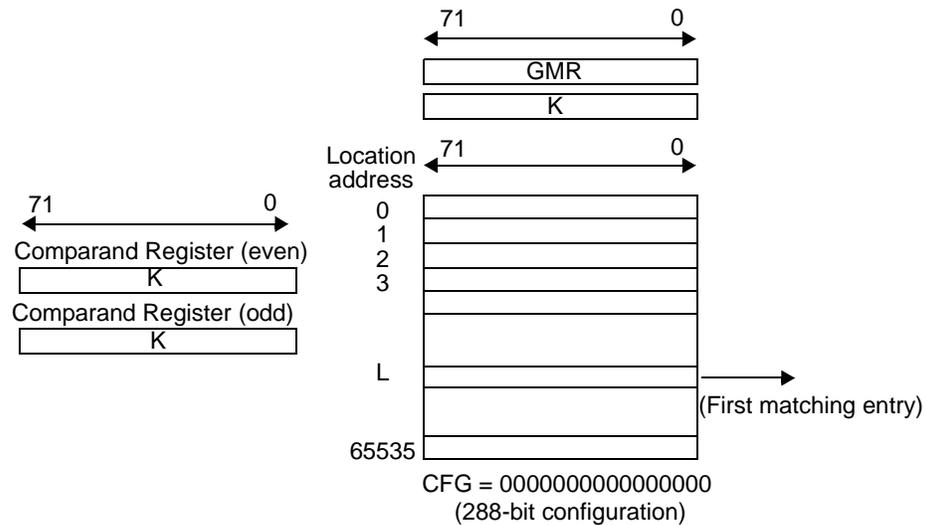
**Figure 10-7. x72 Table with One Device**
