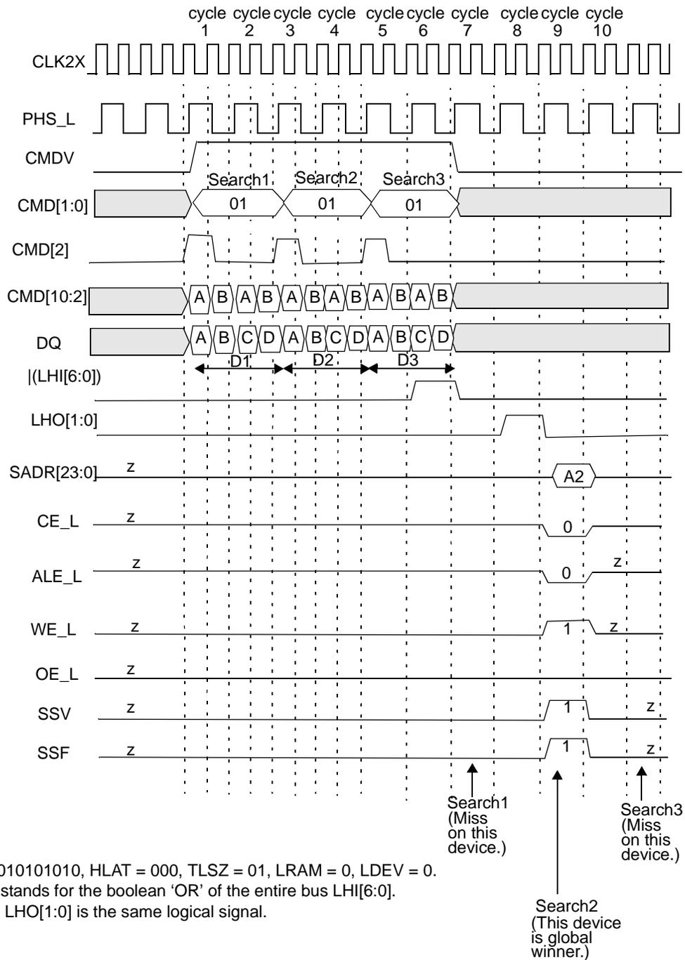
Figure 10-54. Timing Diagram for 288-bit Search Device Number 1
