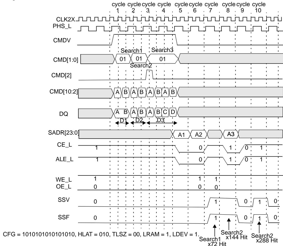
Figure 10-71. Timing Diagram for Mixed Search (One Device)
