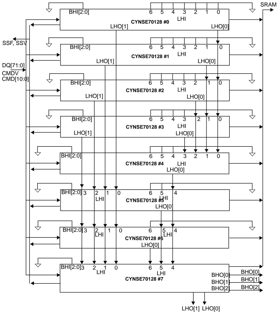
**Figure 12-9. Table of a Block of Eight Devices**
