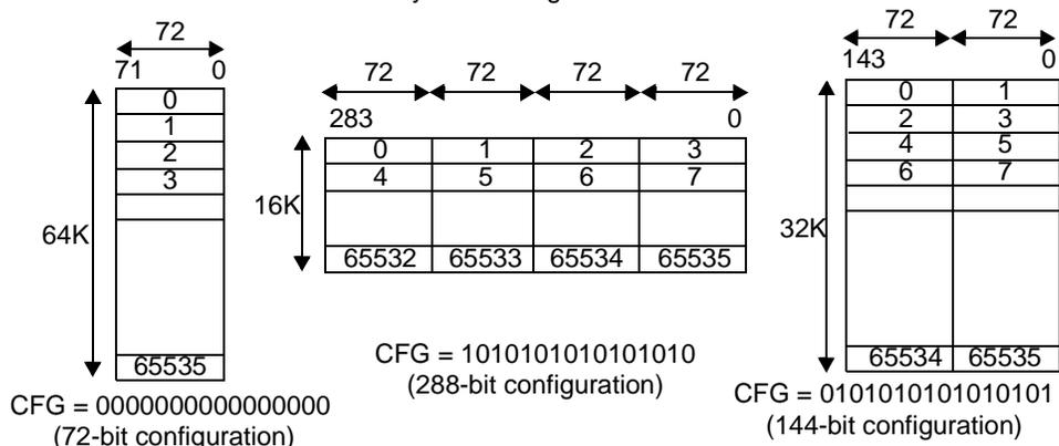
Figure 9-1. Addressing the CYNSE70128 Data and Mask Arrays
