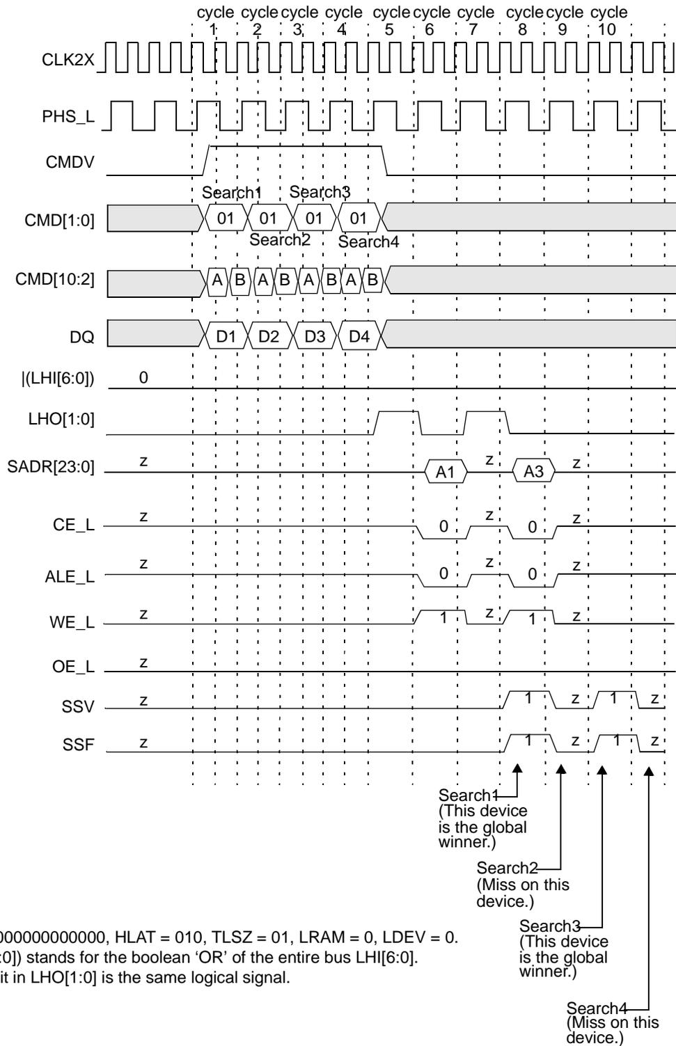
**Figure 10-9. Timing Diagram for 72-bit Search Device Number 0**
