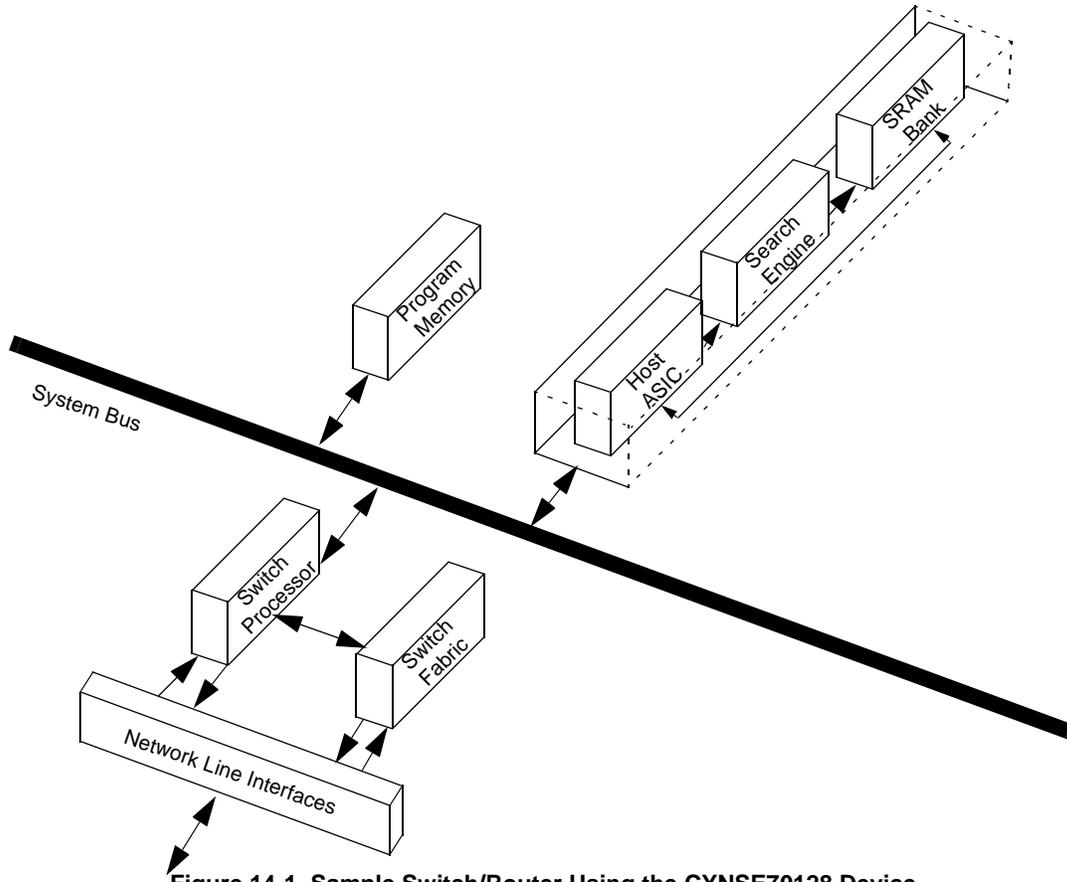
Figure 14-1. Sample Switch/Router Using the CYNSE70128 Device
