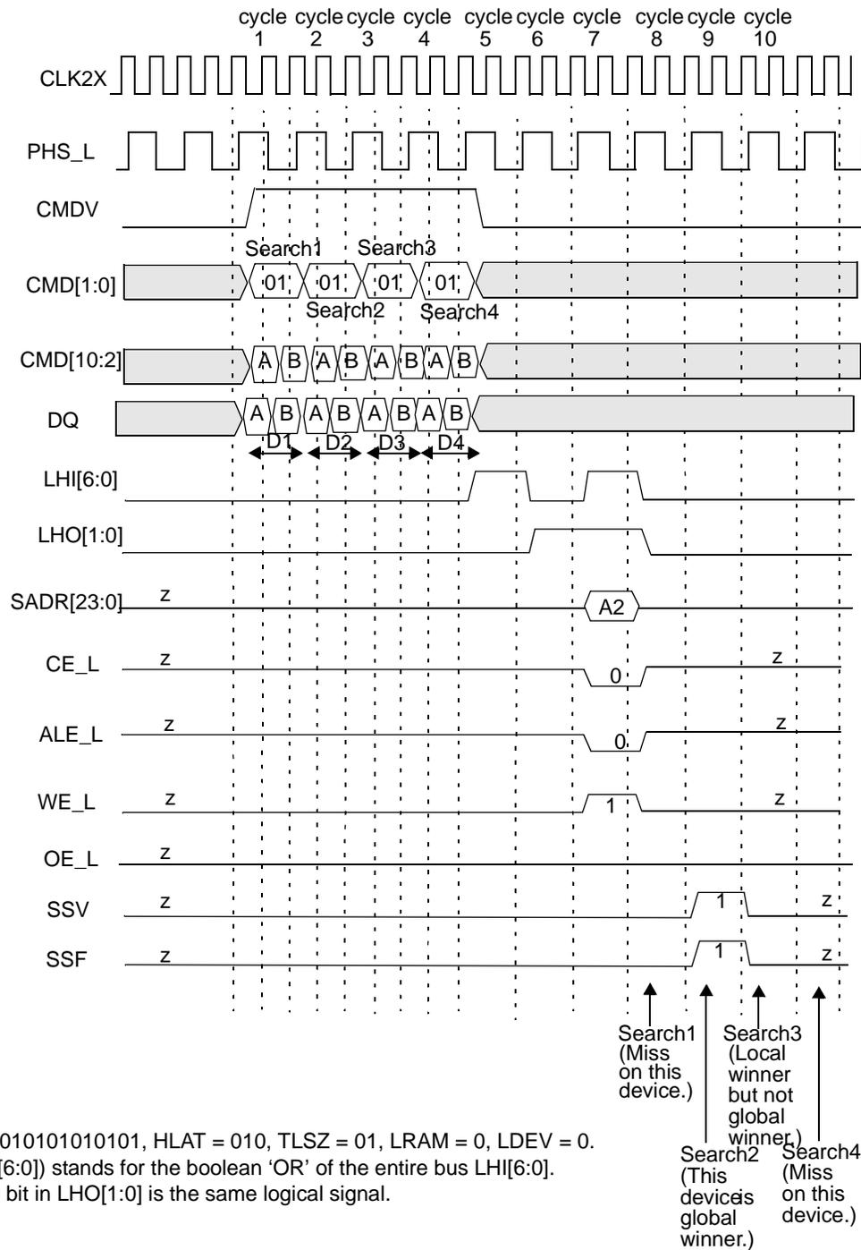
**Figure 10-32. Timing Diagram for 144-bit Search Device Number 1**
