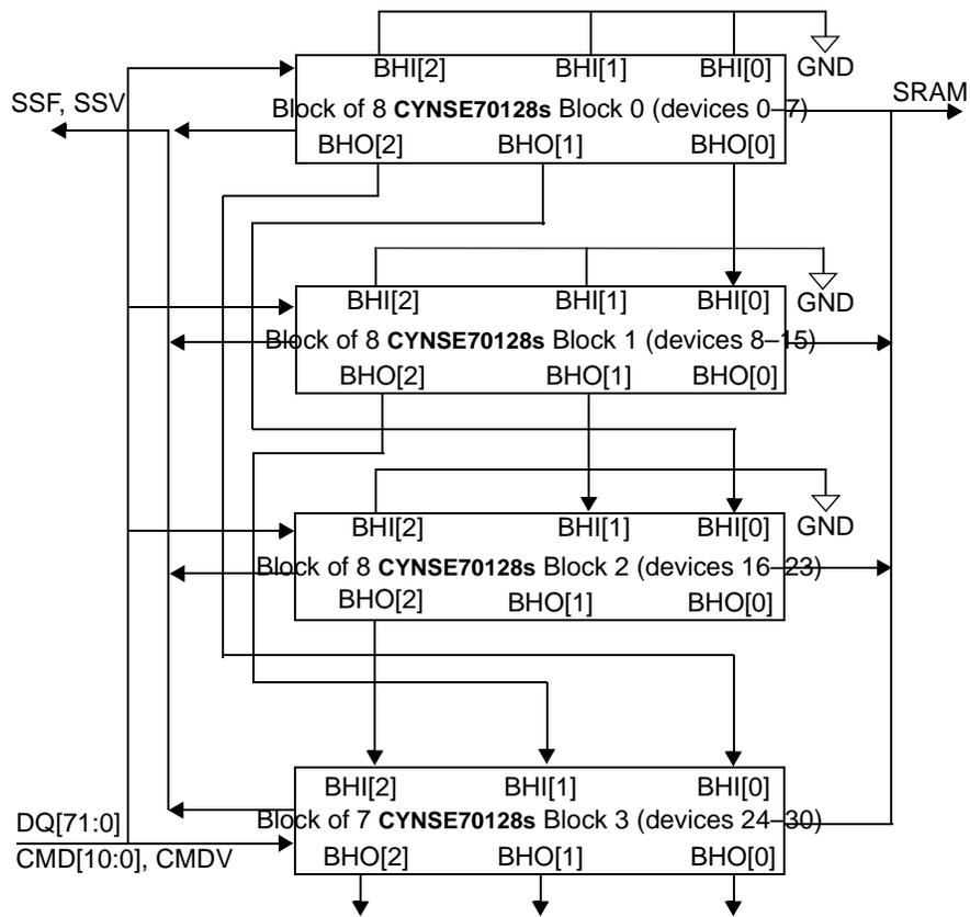
Figure 10-35. Hardware Diagram for a Table with 31 Devices
