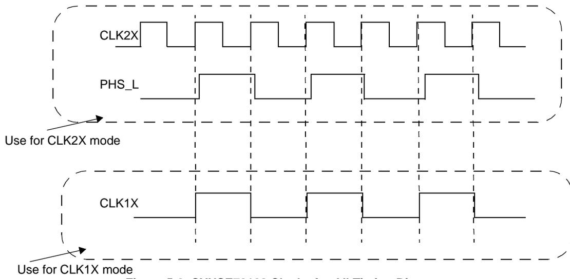
**Figure 5-3. CYNSE70128 Clocks for All Timing Diagrams**
