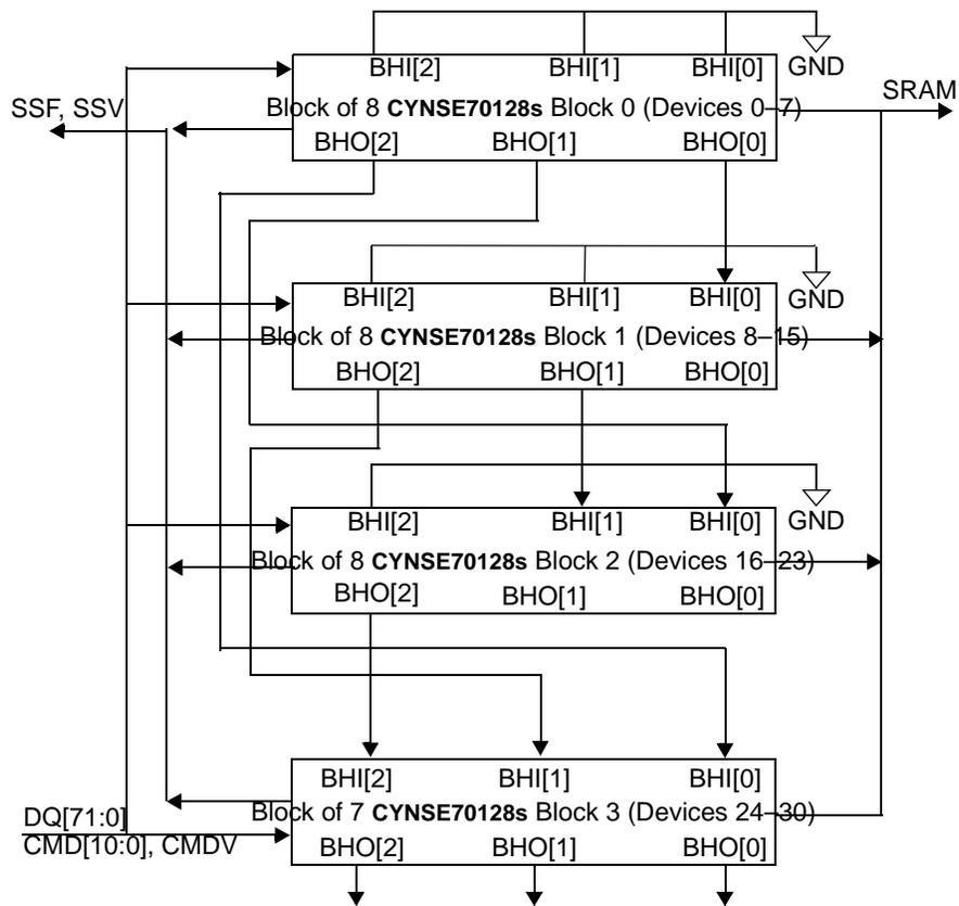
**Figure 10-13. Hardware Diagram for a Table with 31 Devices**
