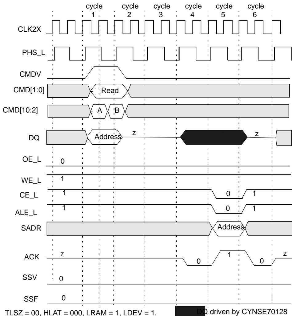
**Figure 12-1. SRAM Read Access (TLSZ = 00, HLAT = 000, LRAM = 1, LDEV = 1)**
