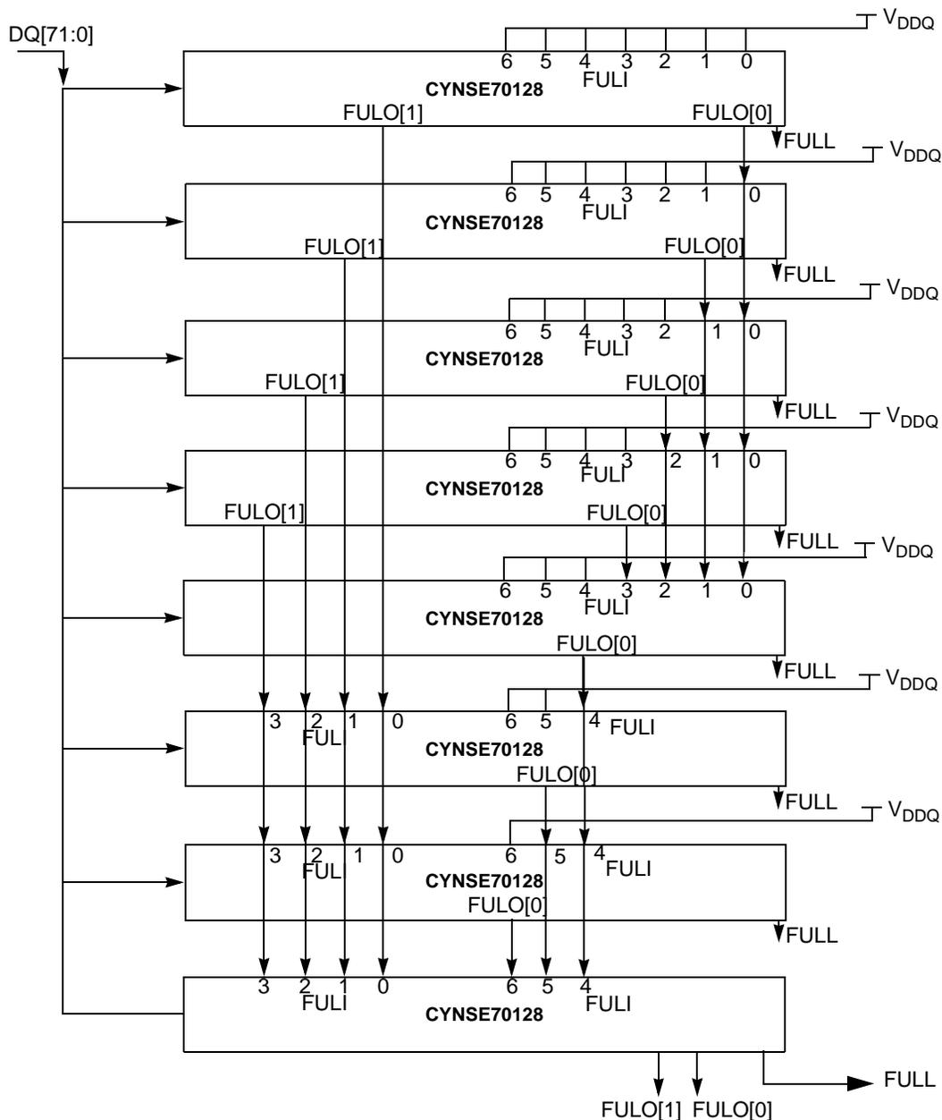
**Figure 11-3. FULL Generation in a Cascaded Table**
