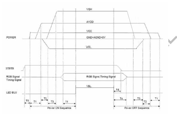
Note: T1≥20ms, T2≥20ms, T3≥5ms, T4≥100ms, T5≥5ms, T6≥5ms.
