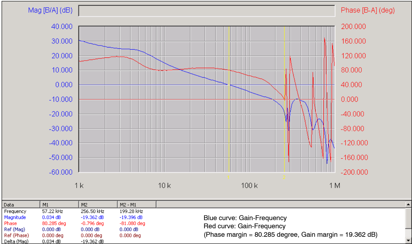
Figure 14. Closed-loop Voltage Loop-gain of the NCP81044
