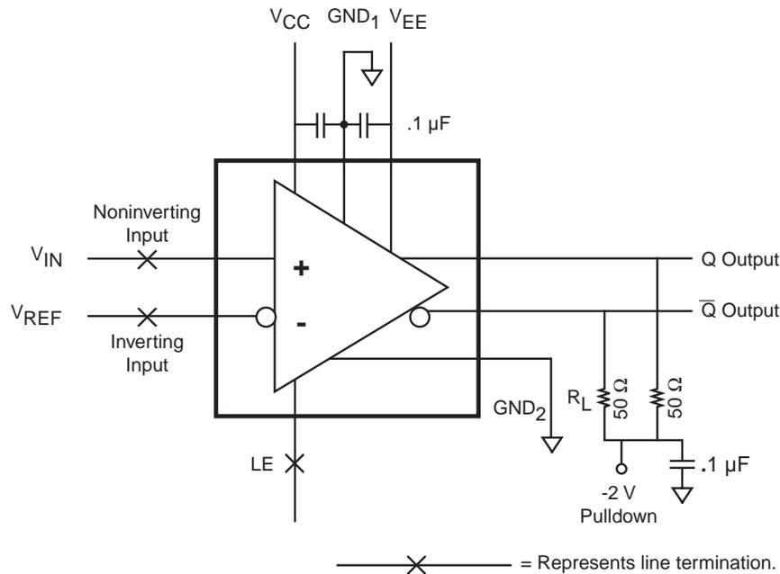
**Figure 4 - Equivalent Input Circuit**
