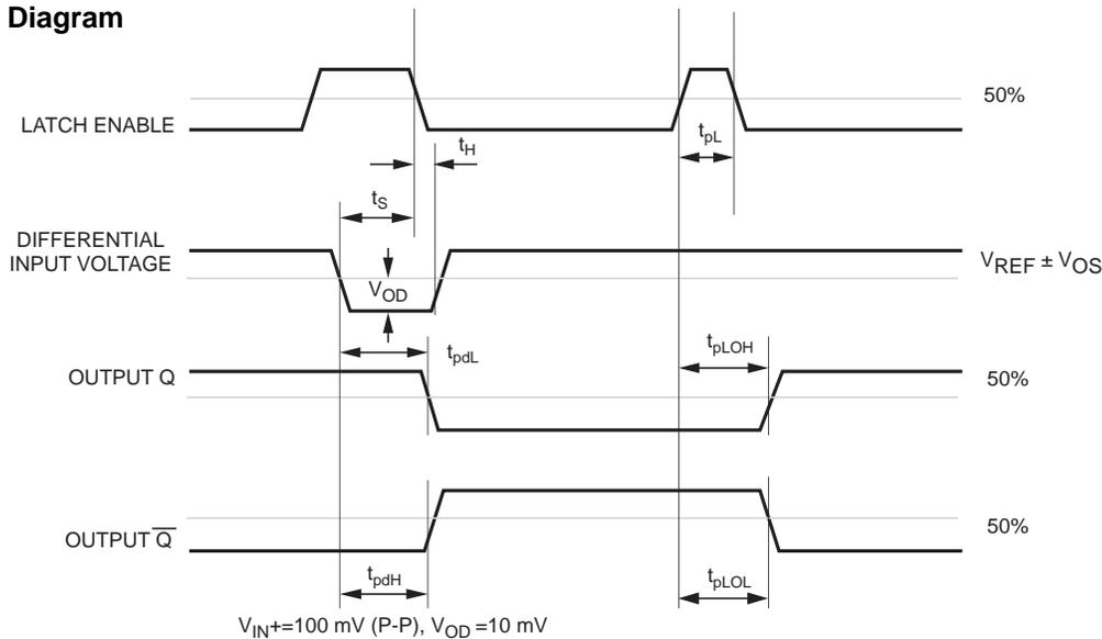
The set-up and hold times are a measure of the time required for an input signal to propagate through the first stage of the comparator to reach the latching circuitry. Input signal changes occurring before  $t_s$  will be detected and held; those occurring after  $t_H$  will not be detected. Changes between  $t_s$  and  $t_H$  may or may not be detected.
