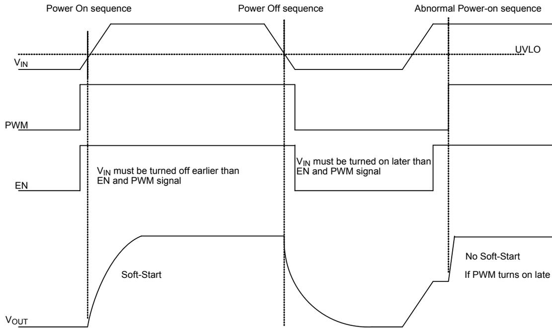
Figure 2. Power On Sequence Control by V<sub>IN</sub>
