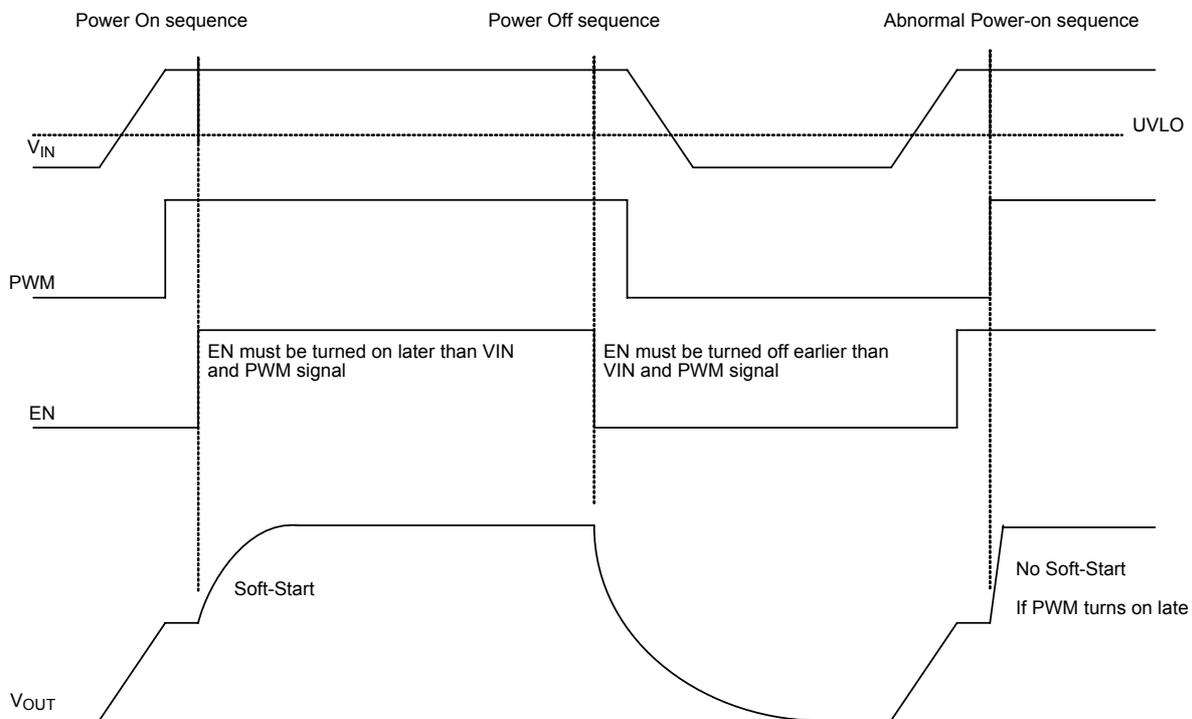
Figure 1. Power On Sequence Control by EN
