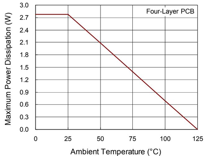
Figure 7. Derating Curves for RT8488 Package
