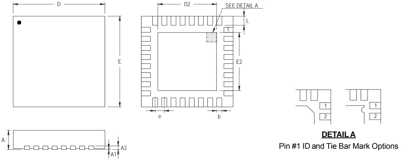
Note : The configuration of the Pin #1 identifier is optional, but must be located within the zone indicated.
