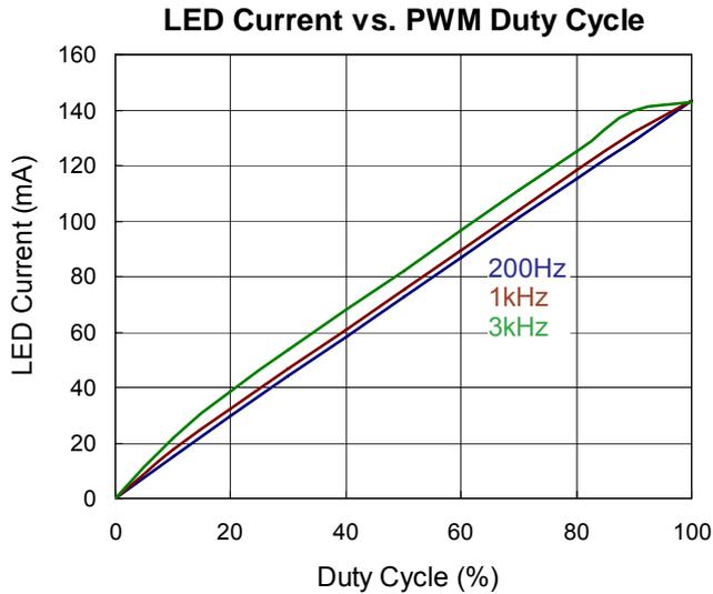
Figure 4. LED Current vs. PWM Dimming Duty Cycle
