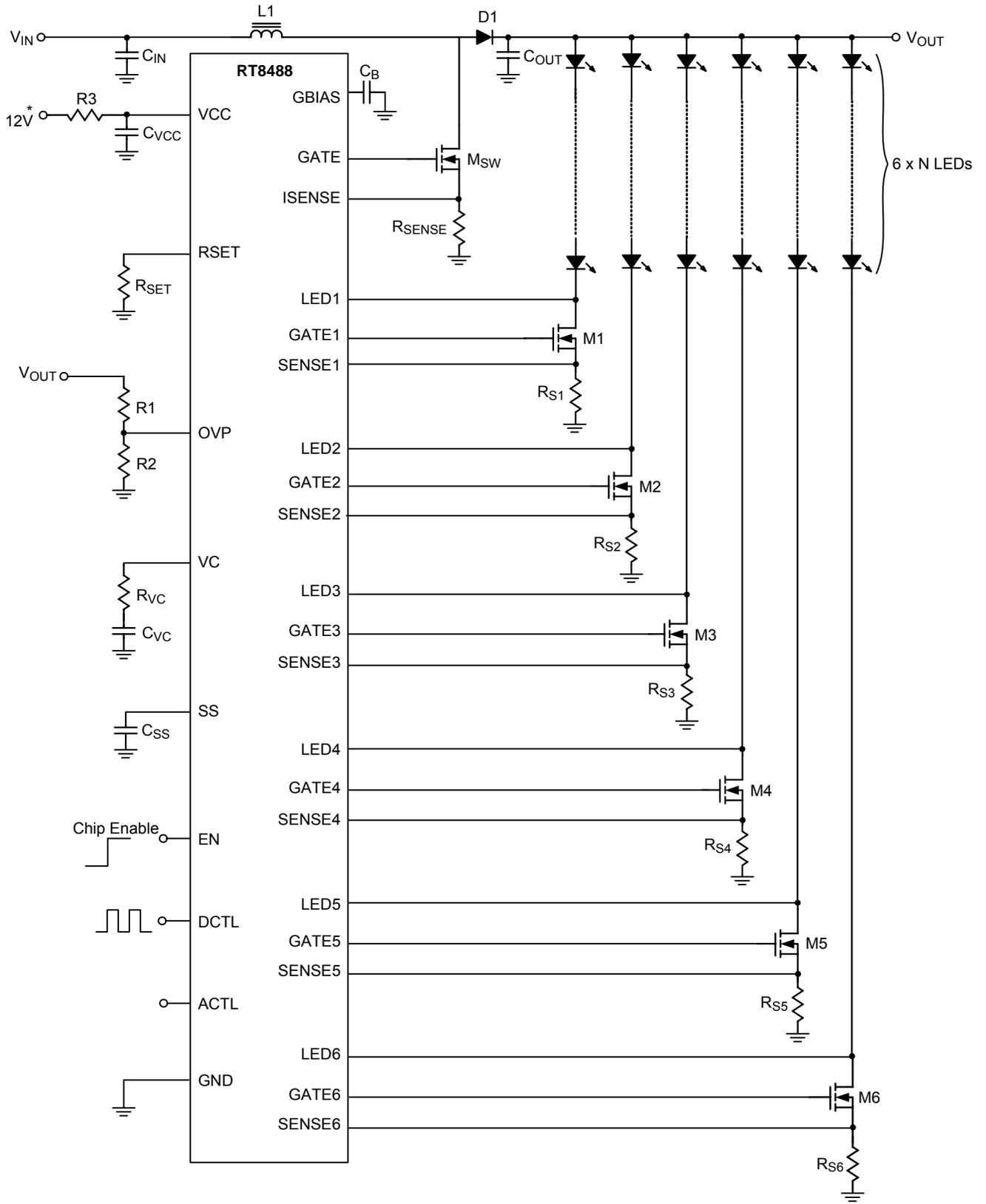
\* : If  $V_{IN}$  is operated above 12V, it is recommended to keep the  $V_{CC}$  at 12V for optimal application
