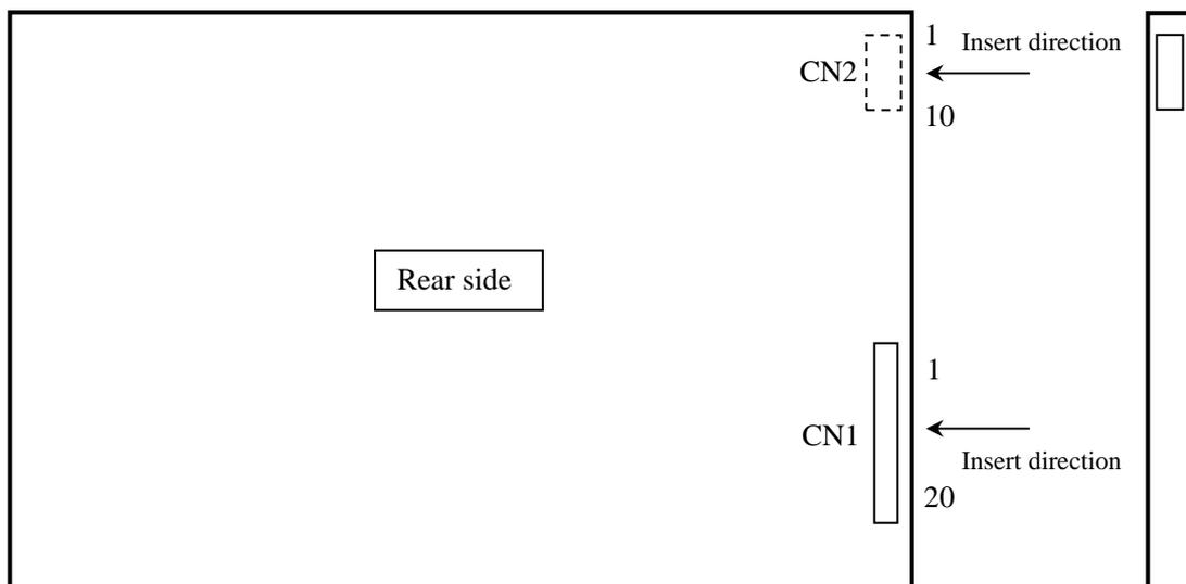
4.5.4 Connection between receiver and transmitter for LVDS
