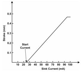
Figure 19. Voice Coil Stroke vs. Isink Current
