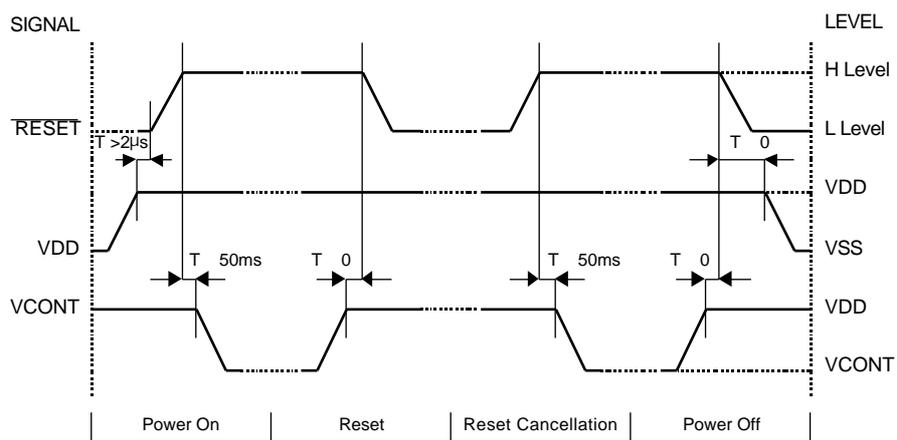
Please maintain the above sequence when turning on and off the power supply of the module. If VEE and/or VCONT is supplied to the module while internal alternate signal for LCD driving (M) is unstable or RESET is active, DC component will be supplied to the LCD panel. This may cause damage to the LCD module.
